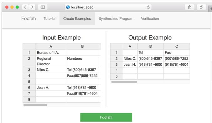
Figure 4: FOOFAH UI for specifying input-output examples
